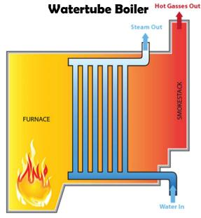
utensils. After the steam is used in processing, it condenses back into water, and that water is often returned to the boiler where it is reboiled, and the process begins once again.
